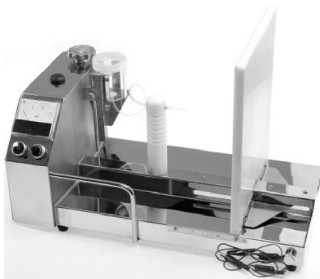
Figure 3 Photograph of Electrospinz Adam Series electrospinning apparatus (microscope not shown for clarity).
